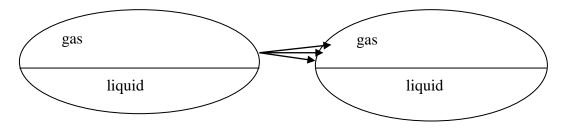
a) The propane leaks from a hole above the liquid surface, and the jet hits the other tank. The hole radius is 0.5 cm. What is the leak rate? Explain your choice of formula..
