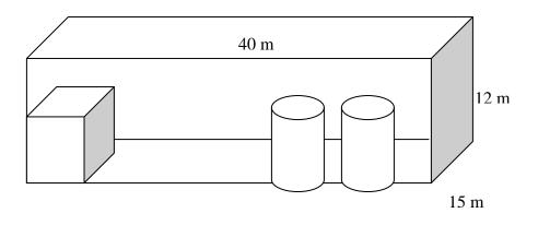
a) What is the volume of the gas cloud? Approximately how large a proportion of the cloud will contribute to overpressure generation in a possible explosion? Where would you locate the ignition point in order to generate as high an overpressure as possible? Give a brief explanation.
