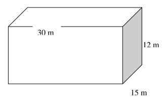
a) How many kg of methane does the gas cloud contain? Where would you locate the ignition point to maximise the overpressure in an explosion? Explain.
