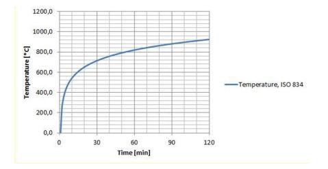
Figure 1: ISO 834 standard temperature/time fire- curve
